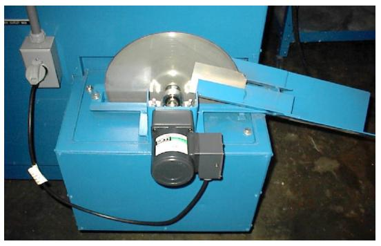
The <u>Replacement Oil Skimmer</u> is a drop in for the old style skimmers taking just a few minutes to install. The easily installed <u>Retrofit Kit Oil Skimmer</u> is for equipment without an existing skimmer. It includes a Skimmer reservoir to be welded to the Cabinet Reservoir, Box Lid, and complete installation instructions.
