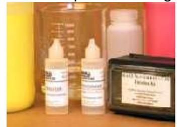
Remember the only way to reliably measure chemical concentration is by titrating. Titrating the cleaning solution on a regular basis determines the amount of cleaning chemical per gallon of water and allows you to decide if additional cleaning chemical is required.
