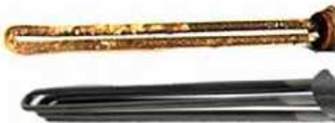
Hard Water scale shown on top heating element can cause early failure. Element on bottom shows no signs of scale.
