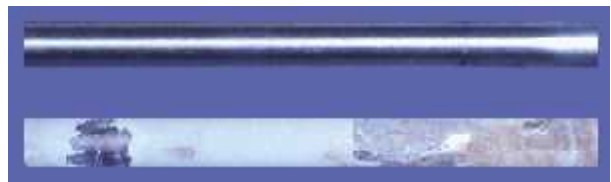
A Clean Stainless Steel electrode and the results of operating the same electrode in scale forming hard water conditions.
