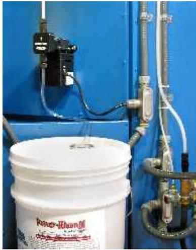
Typical Rinse Chemical Injector pump mounted on STINGRAY® parts washer
