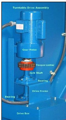
optimum cleaning, it is critical that the turntable rotates during the wash cycle. Check to make sure that the lower part of the turntable drive shaft below the clutch is turning during a wash cycle.
