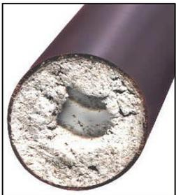
as **scale** or **scum**. These chemical reactions **use up** some of the detergent to form the sludge, reducing the amount of detergent available for cleaning. The sludge is additional waste that must be disposed of from your machine. Scale and scum **do not rinse** away easily. They tend to
