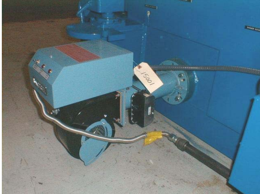
Fig. 0 - 7: Burner Blower Motor (380,000 BTU Burner Shown; Other Sizes Similar)
