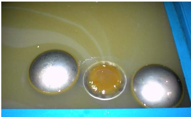
Floating suction device pulls oil from surface for maximum separation
