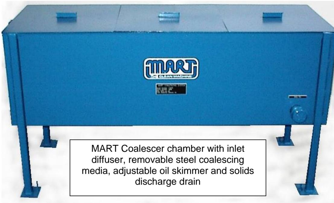
MART Coalescer chamber with inlet diffuser, removable steel coalescing media, adjustable oil skimmer and solids discharge drain
