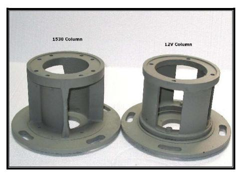
The 1530 Column versus the 12V column. Note the stiffener ribs on the 1530 column and the smaller amount of open area. (Left 1530, Right 12V)
