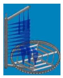
As the Turntable rotates, the C-PBM. shaped blasting from the top down, bottom upwards and across the cabinet, pivots on its vertical axis. making 46degree sweep and return, every fifteen seconds. throughout the wash cycle. The speed of the
