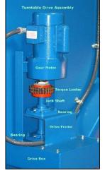
optimum cleaning, it is critical that the turntable rotates during the wash cycle. Check to make sure that the lower part of the turntable drive shaft below the clutch is turning during a wash cycle.
