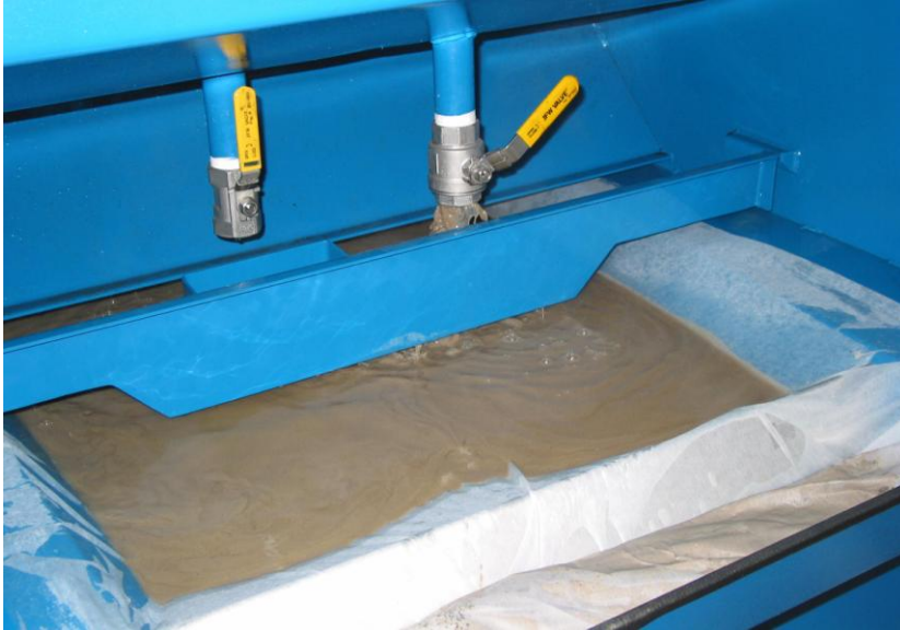
Draining encapsulated waste onto the filter paper
