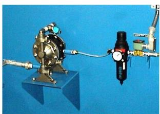
Variable speed Stainless Steel Pump System transfers solution from Washer to Oil Coalescing Chamber
