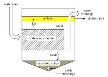
Although the stem is highly effective while the wash machine is in use, the coalescing efficiency is improved during periods when solutions are cooler such as non-production hours. Non-emulsifying cleaners must be used to maximize the advantages of coalescer technology.
